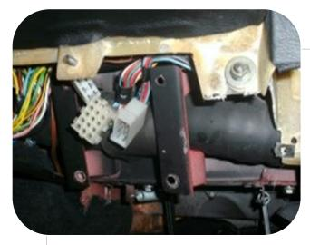
Step 10. Remove the original mounting brackets on both sides.
