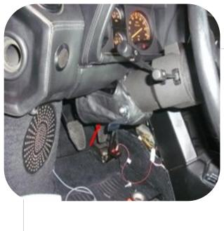
Step 4. Remove the leather protection from the steering column.
