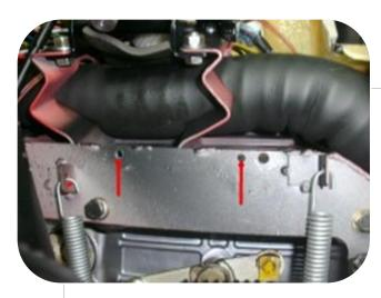
Step 13. Drill 2 holes to fit the ECU. Use the ECU as a template.
