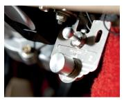
Left: electric motor attaches to a new part in the column. Above: dial allows amount of assistance to be tweaked
